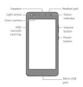
Do not cover the light sensor, as this will affect some of the phone's functions. Ensure that you use a screen protector that has a purpose-built hole for the light sensor.
