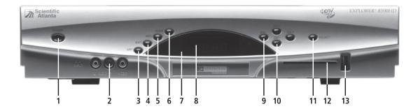
**1** Power Provides power to the unit. The 😃 symbol appears in the upper right portion of the display when power is on.
